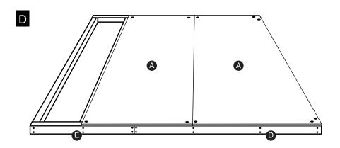
Nails every 12" (30 cm) through Floor Panels into all Floor Bond Boards and Joists
